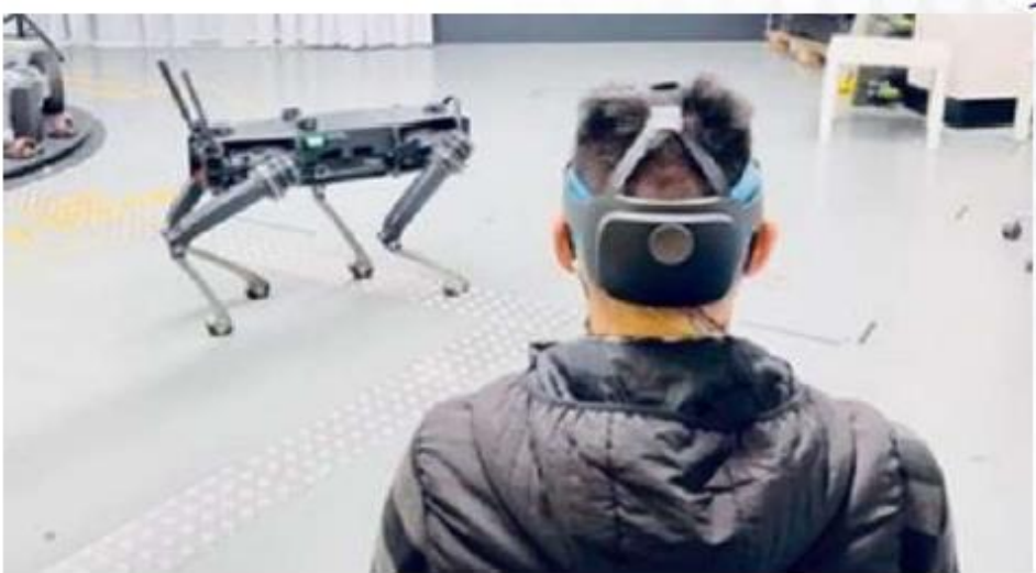
A new sensor design used to control a robot using brain waves
